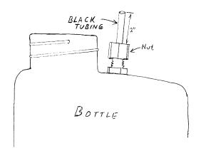
direction. Allow about 2 feet (60 cm.) extra for slack. Label both ends of the tubing with the chemical name. Slip one end over the proper tube and the other end over the exposed black tubing of the solution bottle. The 5 gal. water bottle connects to the WATER (#5) tube.
