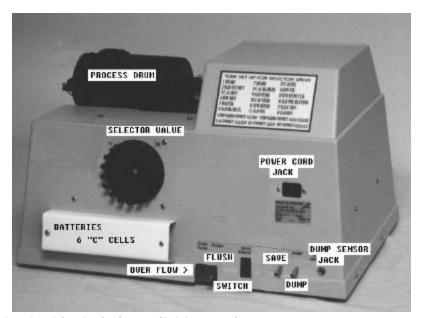
jack on the back of the unit. If a plumbed-in drain is available, use it.
