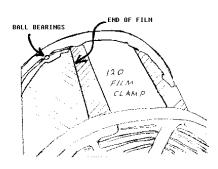
120/220 FILM. Separate the tape from the backing paper and fold it back over the film. This will stiffen the end of the film. Load the taped end into the reel. Feed until the back end is passes the ball bearings.
