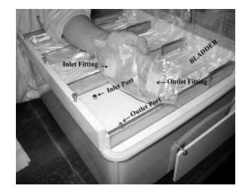
Mount the BLADDER by pushing the INLET and OUTLET FITTINGS down and twisting back and forth on the INLET and OUTLET PORTS. Slip the other end of the bladder under the white rod and lay over the bottom part of the bladder. If you are not using all 3 BLADDERS you must cover any open PORTS with a plug.
